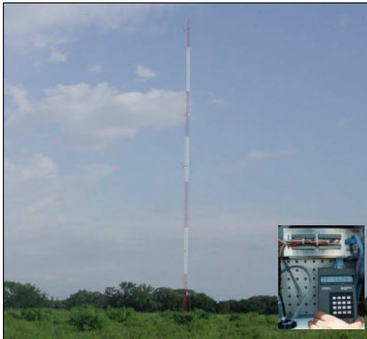
Reference station for wind resource evaluation
