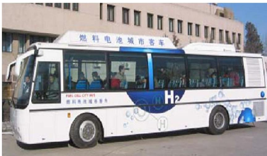
Figure 4 - The Dalian Institute of Chemical Physics (DICP) unveiled this hybrid fuel cell bus (30 kW fuel cell) in December 2002.
