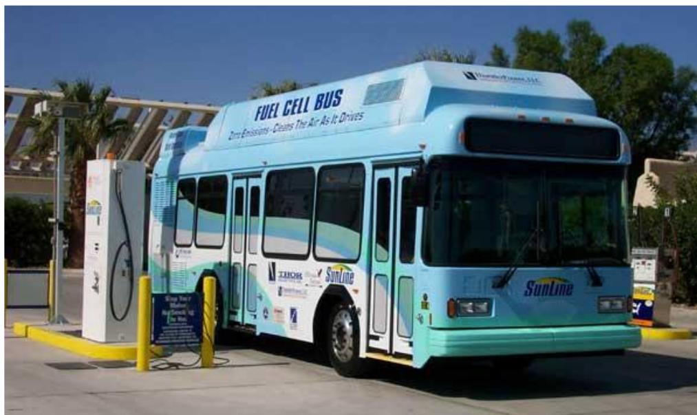
**Figure 2 - The Thor Industries ThunderPower bus with a UTC fuel cell engine was operated in revenue service in 2003 at Sunline Transit in Thousand Palms, California**
