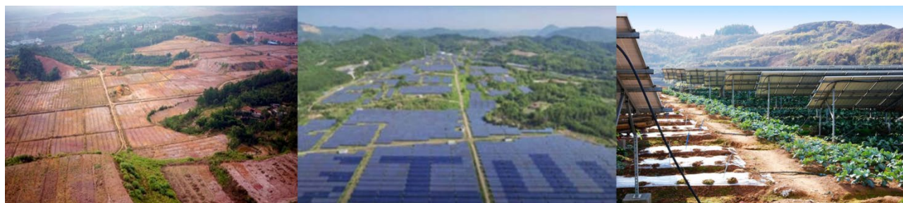
The agrivoltaics park in Jiangshan, China, before(left) and after (center, right) installation. Source: Xiao and others. 39
