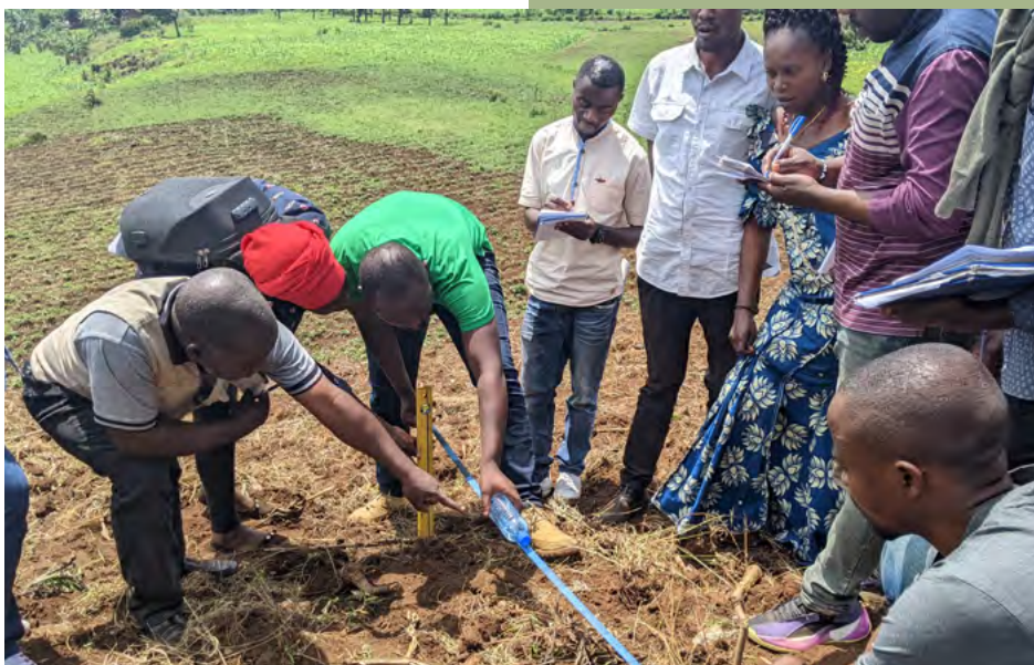
Implementation of erosion control as a restoration option, pictured here in Mulungu, determining the slope of the land with local materials (used water bottle).
