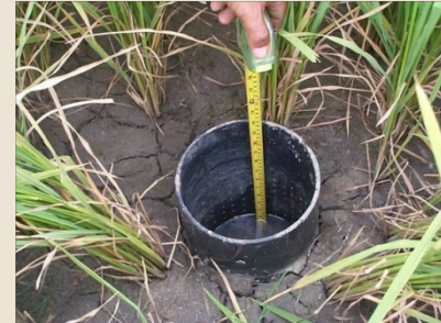
Perforated tube for observing water level in the soil
